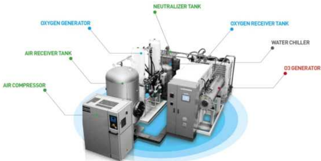
[Fig. 41] General system configuration of Ozone system
