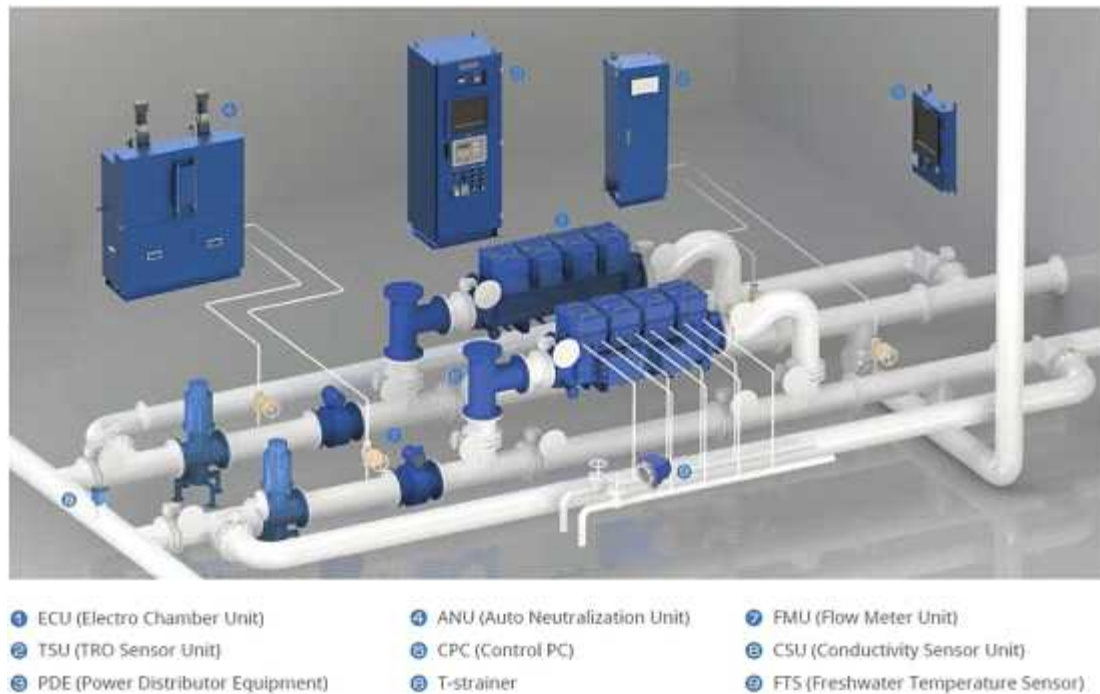
[Fig. 5] General arrangement of ballast water management system using full flow electrolysis technology.
