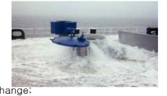
2. Flow-through method – a process by which replacement ballast water is pumped into a ballast water intended for the carriage of ballast water, allowing water to flow through overflow or other arrangements;
