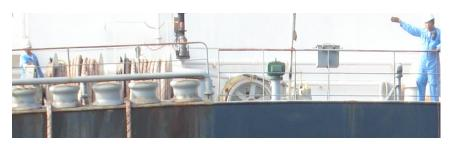
mooring line some elasticity. However, due to the limited elasticity present in a wire or wire and rope tail mooring line when compared to the elasticity of a synthetic line, it is recommended that wires are not run as the first lines when coming alongside to heave the vessel into position.
