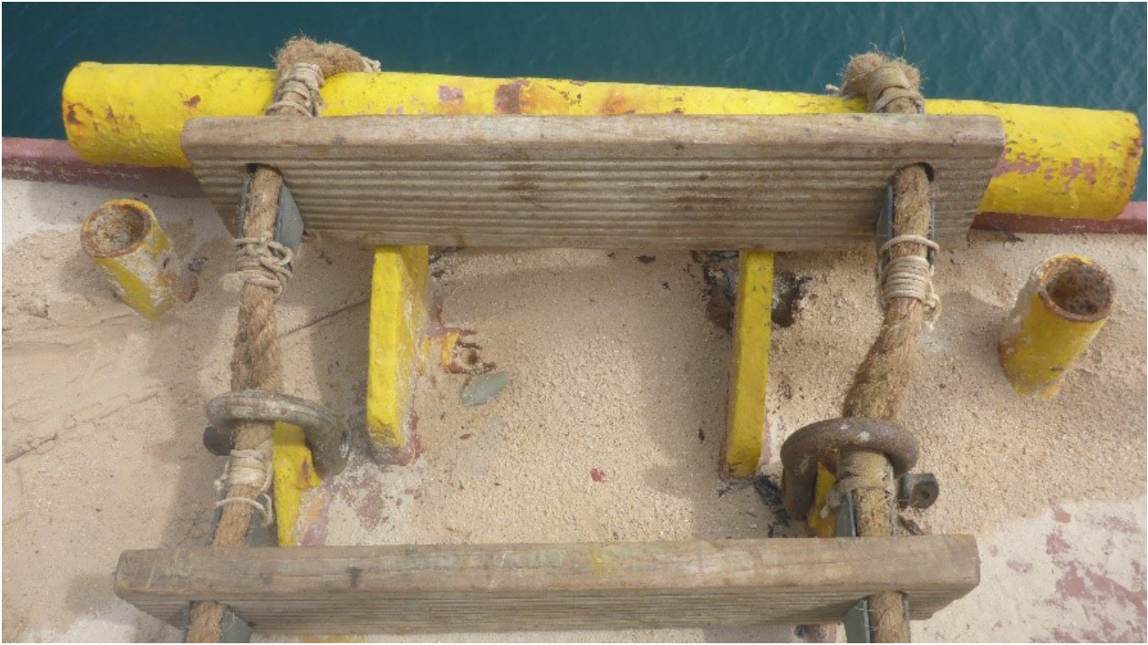
Figure 1. Pilot ladder incorrectly secured to the deck using D-shackles to choke the side ropes.
