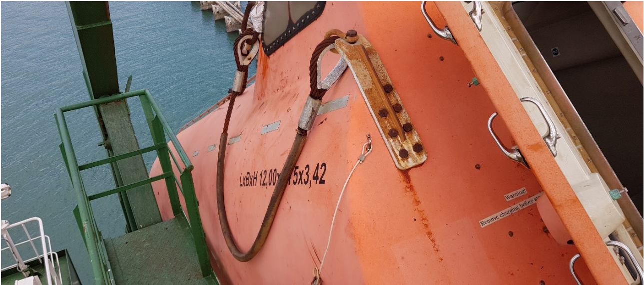
Figure 1. Lifting sling encased in plastic sheathing
