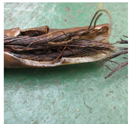
Figure 3. Lifting slings parted due to undetected corrosion.
