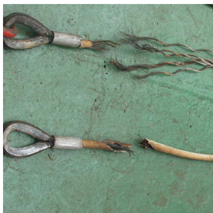
Figure 3. Lifting slings parted due to undetected corrosion.
