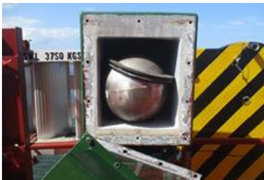
Gasket slipped off
